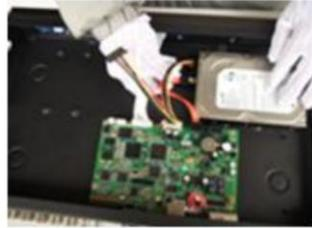
②HDD data line and power line connection
